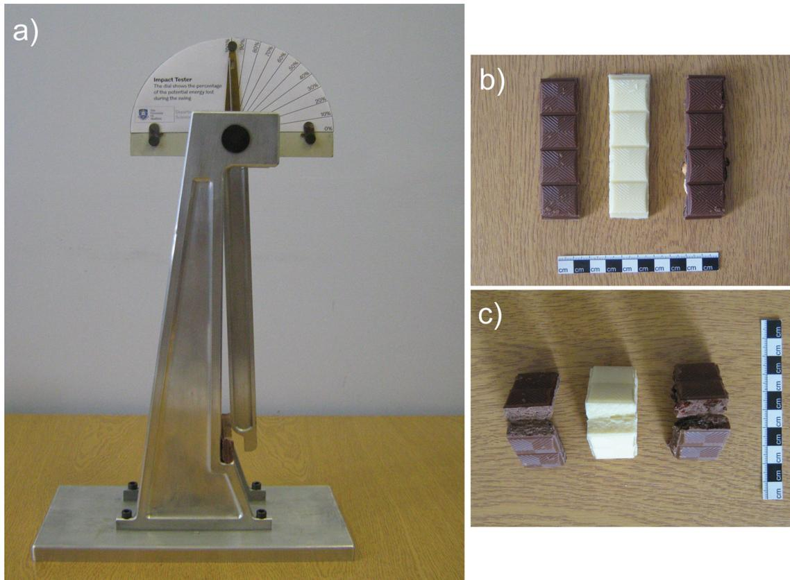
Figure 3 – a) Image of the rig produced for this work, with a sample in the test position (the rig pendulum is 30 cm long). b) Suitable segments of chocolate bars that can be used as specimens (milk, white and fruit and nut chocolate respectively). c) The same samples after testing, positioned to show their fracture surfaces (energy absorbed in these tests were: milk 77%, white 85% and fruit and nut 55%).
