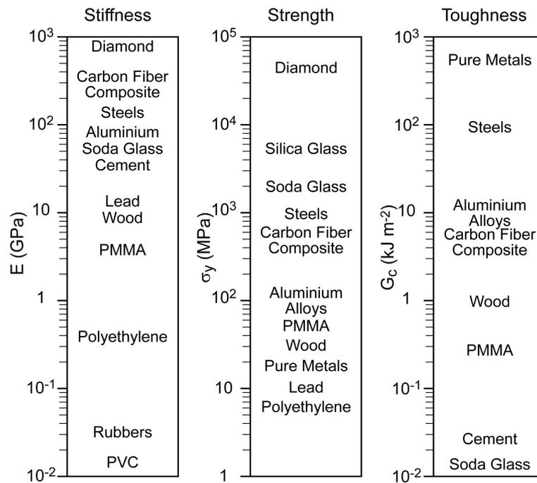
Figure 1 – Approximate ranking of different common materials for stiffness (Young's modulus,  $E$ ), strength (yield or fracture stress,  $\sigma_f$ ) and toughness (Critical strain energy release rate,  $G_c$ ) Adapted from [1].
