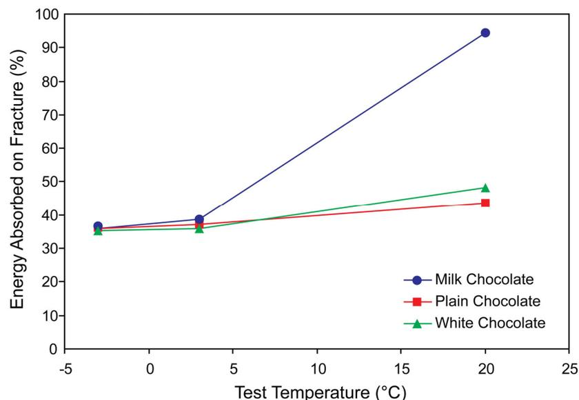
Figure 4 – Energy absorbed on fracture at different test temperatures for different types of chocolate.
