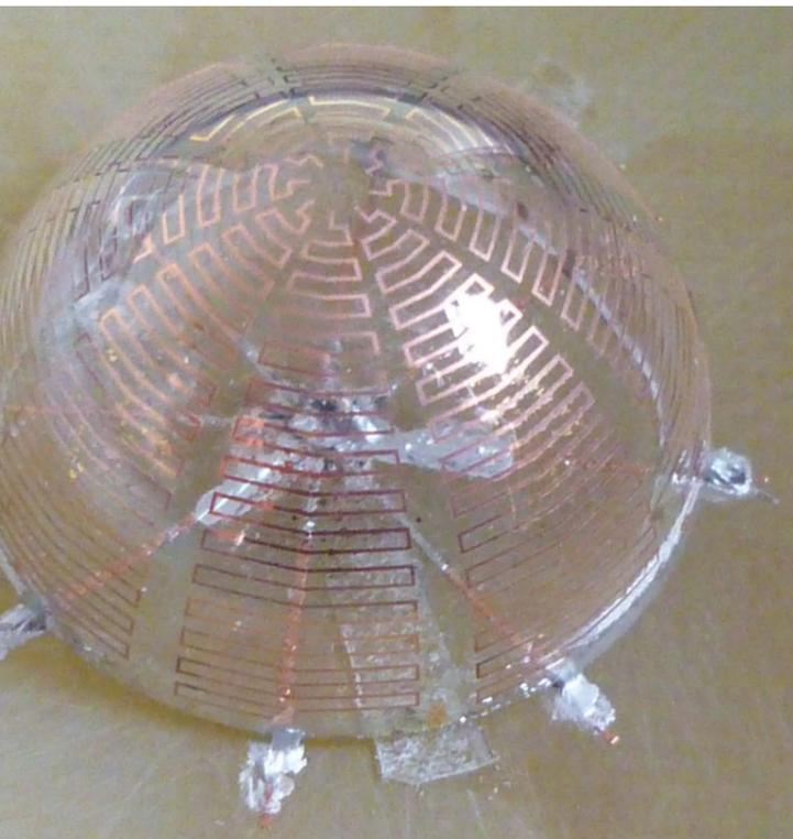
3D photolithography has the potential to displace existing sequential direct-write techniques and enable new product designs.
