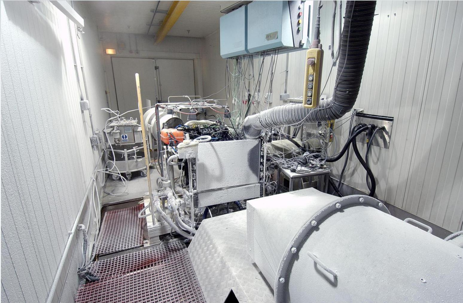
Dynamic dynamometer encapsulated test facility – can provide efficient, cost effective and realistic testing on a rig as opposed to building expensive prototype vehicles, which require specialised vehicle-based test facilities or testing in remote cold climate locations.
